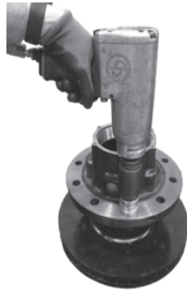
Figure 16: Stud draw-in process
