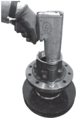
Figure 16: Stud draw-in process
